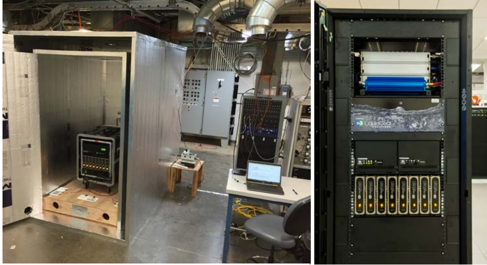
Figure 3. Eight servers instrumented at NREL's Advanced HVAC Systems Laboratory in Golden, Colorado (left) and eight servers installed at NREL's ESIF data center in Golden, Colorado (right) Photos by Eric Kozubal and Dennis Schroeder, NREL
